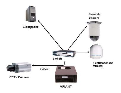
The diagram above shows a simple installation of an AFIANT hybrid. In this example the FleetBroadband Terminal is connected to the network switch, as is the network camera. The CCTV camera is connected directly to the AFIANT hybrid. The computer in this case is a local monitoring and is therefore connected to the switch also. For remote monitoring you would us any computer which had a connection to the internet.
