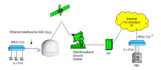
The above diagram illustrates a compressed voice connection over a FleetBroadband ground station FleetBroadband link.
